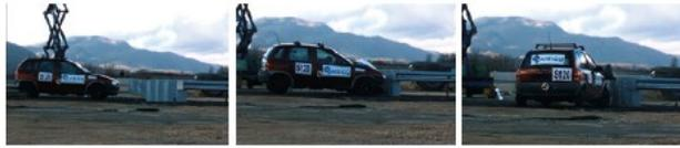
**TT 1.3.110** - Frontal, 0°, no eixo - 1500Kg - 110Km/h (EN1317:4,7)
